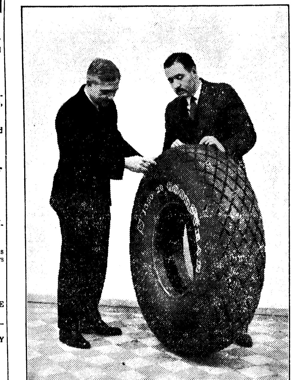
C. C. Slusser and R. S. Wilson, vice-presidents of Goodyear, are shown above with the largest bal- loon truck tyre ever manufactured. The new tyre is a 13.50-20 for truck and bus, designed for air pres- sure of 95 pounds.
